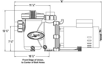
**Note:** When installing the pump, leave a minimum of 2 feet of clearance above the pump for removal of strainer basket.
