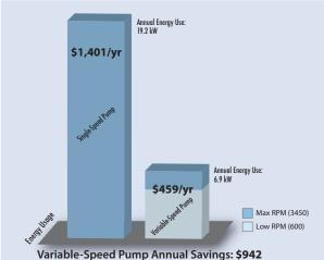
Yariable-Speed PLUMP Annual SavIngS: S942 ased on national average of 50.20/KWh. Rates may vary. Single-speed pump annual costs based on 8 hr. daily run time at max RPV midble-speed pump annual costs based on 2 hr. run-time at max RPM / 20 hrs. at low RPM.
